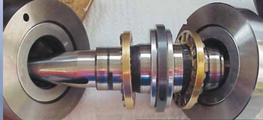
FE8 roller bearing test (non superato)
